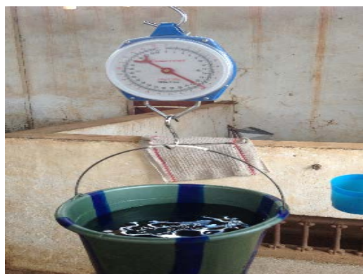
Photo 5: Peson Constant Hanging scale 25 kg
